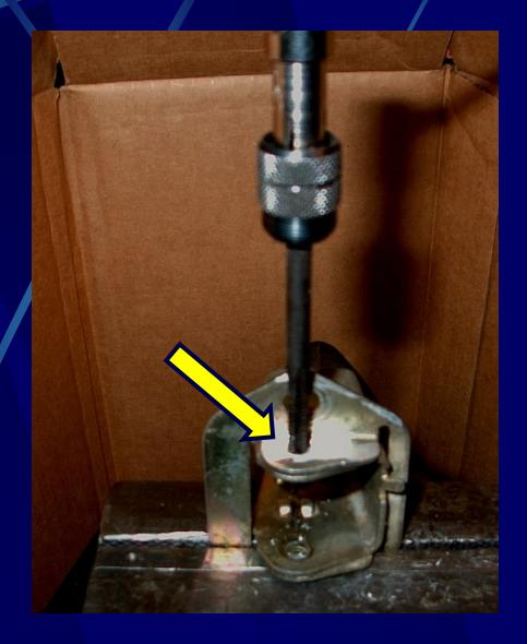
Note that the new latch claw has a small brass bushing in the hole for the spring to pass through. Detach the spring end from the old claw and attach in the same way.
