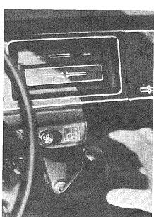
Gear shift lever protrudes from under the dash. Location makes good sense with engine, transmission and differential in a self-contained unit up front.
