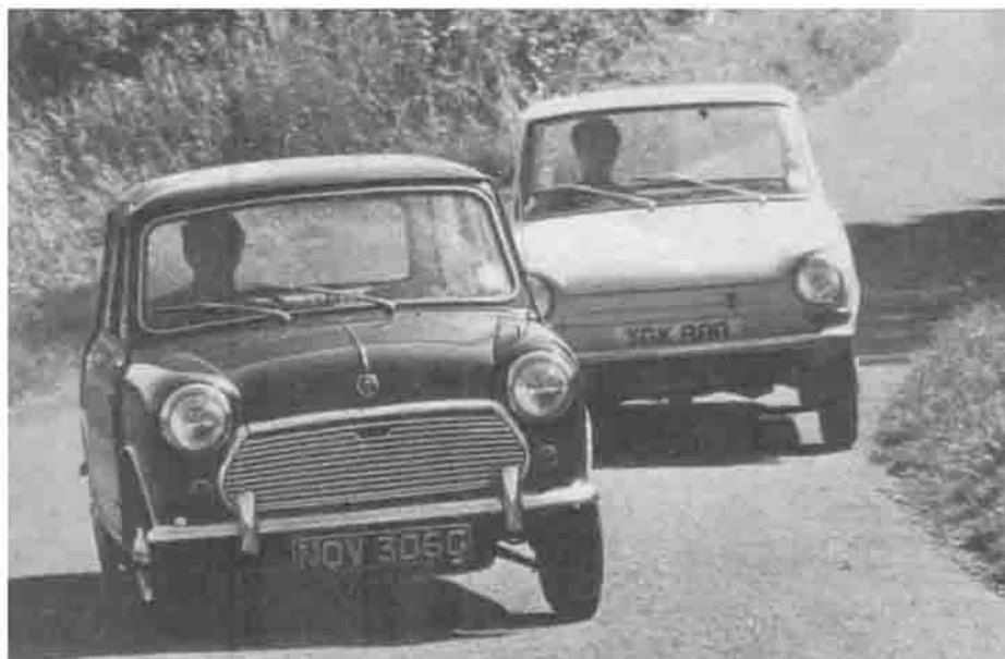
Mini and Daf 44 showing about the same amount of roll under quick cornering.
